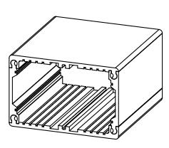
The AE Products Extruded Housings are four panel, interlocking aluminum boxs with end caps. They come equipped with circuit board slots, can be anodized in different color options and cut to lengths up to 72".
